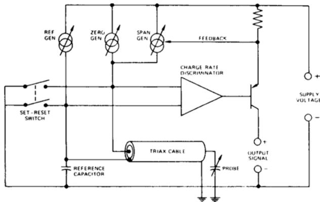
Connected directly across both capacitors is the "charge rate discriminator" amplifier which produces a voltage output when the charging rate of the probe capacitor differs from that of the reference capacitor. When a change in probe capacitance occurs (due to a change in process level), the discriminator amplifier causes an output signal change, which, with voltage feedback, readjusts the probe charging rate through the span generator until the charging rates are again equal.
