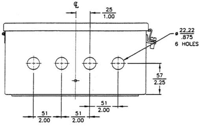
MOUNTING DIMENSIONS FOR 158A LARGE WEATHERTIGHT ENCLOSURE WITH INDICATOR
