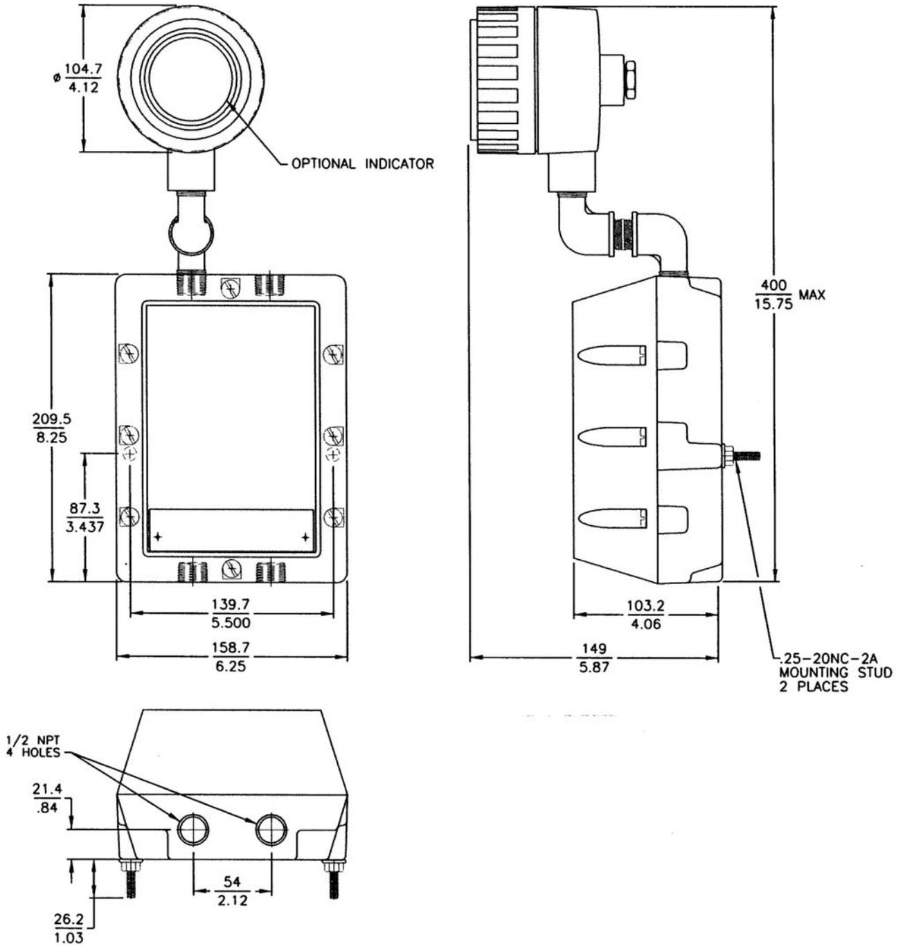
MOUNTING DIMENSIONS FOR 158A EXPLOSION PROOF ENCLOSURE WITH AND WITHOUT INDICATOR
