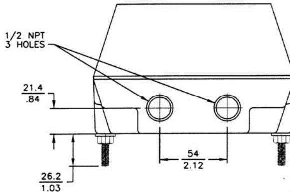
DIMENSIONS OF PROBE MOUNTED CONDUIT
