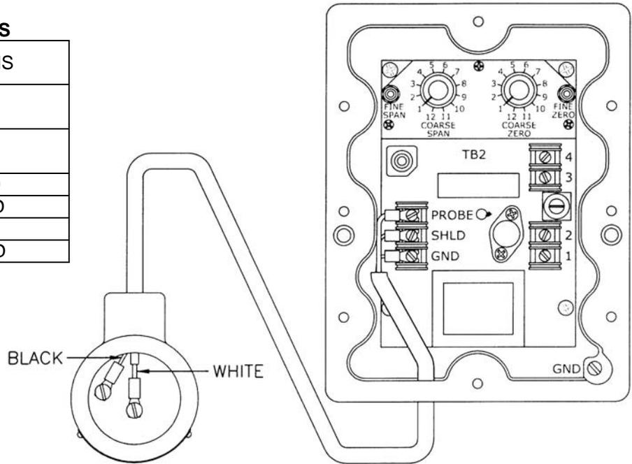
ELECTRICAL CONNECTIONS FOR WEATHERTIGHT AND EXPLOSION PROOF ENCLOSURES
